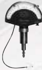
Millimetre Dial Comparator - Built in 1937. The first indicating unit for reliably recording dimensional differences down to 1/1000 mm
