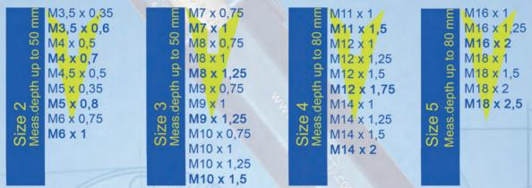
DIN-standards for threads: DIN 2282 (GO) and DIN 2284 (NOGO)
